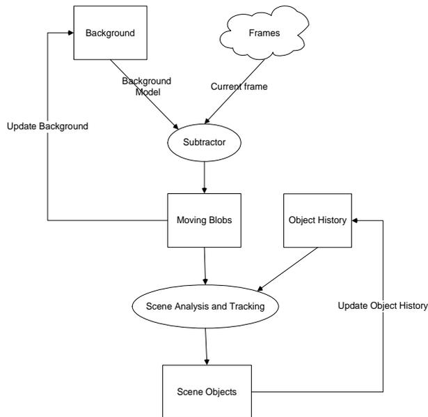
Figure 1 Tracking System Architecture
